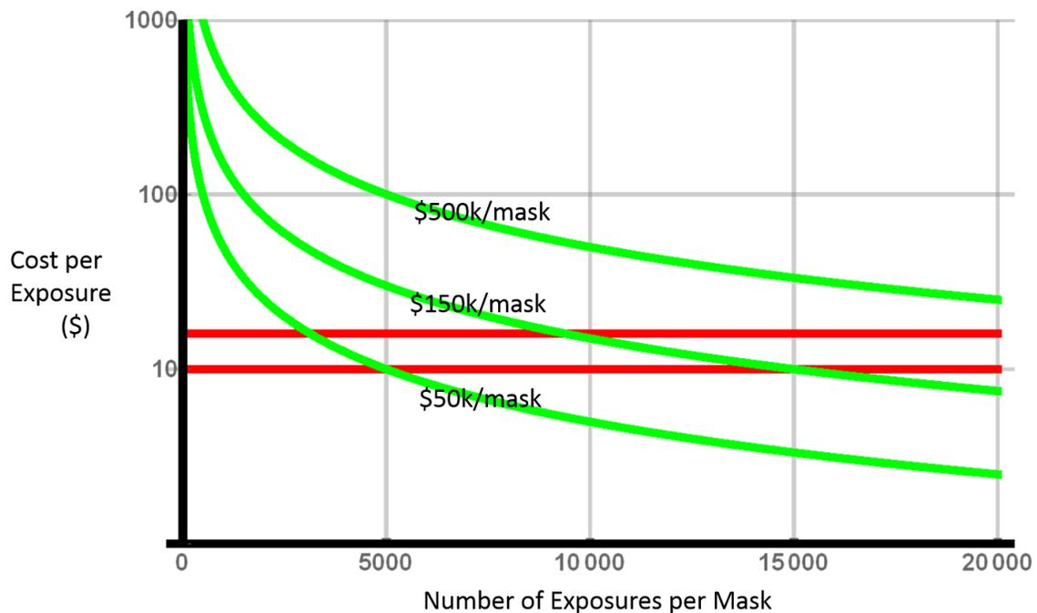
**Figure 3:** Result of the simplified COO model from Sematech for various technologies.<sup>1,2,3</sup> The two horizontal red lines indicate the range of amortized tool cost per full-wafer exposure, \$10 to \$16, as discussed in the text. For low mask usage, i.e. less than a few 1000 wafers/mask , the cost of the masks far outweighs the cost of the litho
