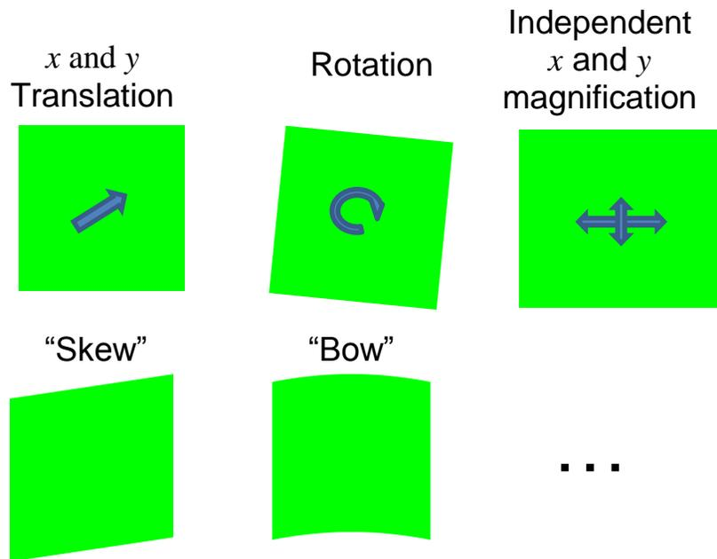
**Figure 4:** Some low order alignment/distortion terms that are automatically sensed and corrected for by the litho tool. Each green “square” represents a single  $\sim 26$  mm X 32 mm exposure field on the 300 mm diameter wafer.
